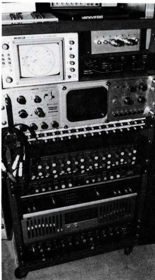
Mini-rack with victroscope, WFM, digital reverb, proc amp, patch panel, parametric equaliser, compressor, expander, graphic equaliser, spring reverb, aural exciter.
